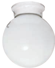
6" FLUSH (BALL) with Pull Chain Switch (1) 60W A19 max. / Medium Base Dimensions: Dia. 6", Height 7.25" CUL damp location
