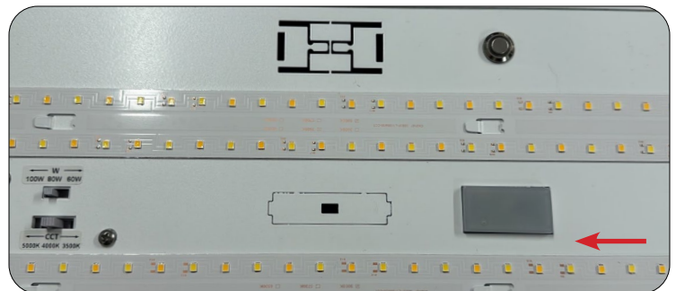
8. Close up the fixture, verify sensor is secured, then proceed to sensor commissioning.
