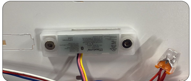
6. Ensure sensor is secured with attached magnets.
